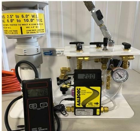
5. Record highest vacuum achieved before PV valve “cracks”. Repeat steps if necessary to record the average number on the form that is used to record results.
