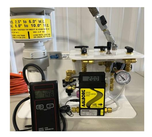
Must measure between -6.0" and -10.0" w.c. to pass
