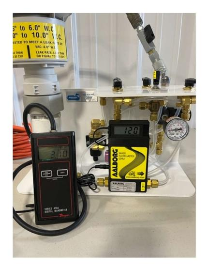
Must measure between 2.5" and 6.0" w.c. to pass
